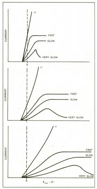
Figure 10. Idealized i-E Curves Modified by MTR with (a) Fast, (b) Slow, and (c) Very Slow Electron Transfer Rates.
