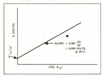
Figure 4. Plot of Potential Versus Log ang+.
