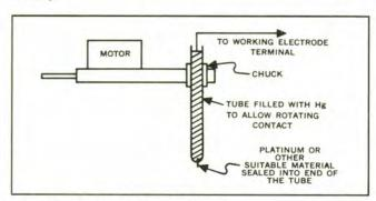
Figure 20. Rotating Electrode Assembly.
