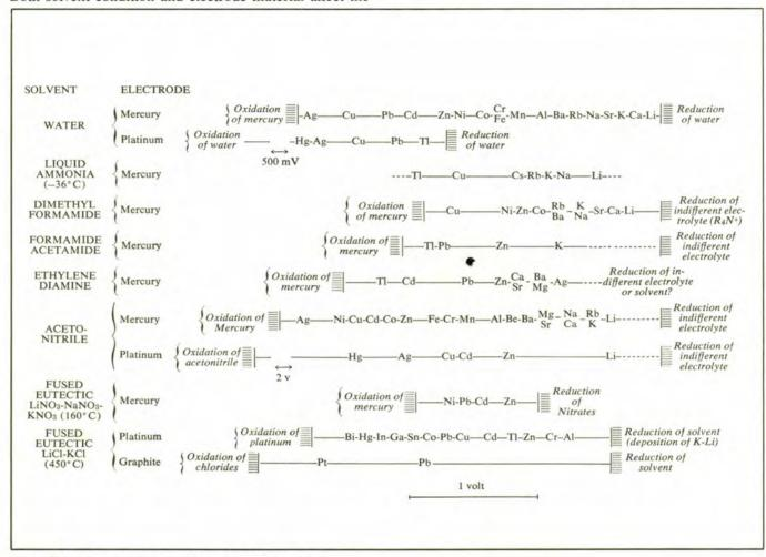
Figure 14. Ranges for Solvent-Electrode Combinations.1
