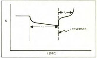
Figure 33. Current Reversal Chronopotentiometry.
