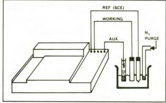
Figure 31. Instrumental Configuration for Chronopotentiometry.
