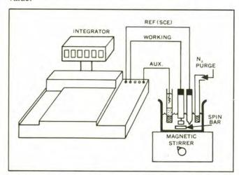
Figure 29. Instrumental Configuration for Controlled Potential Coulometry.
