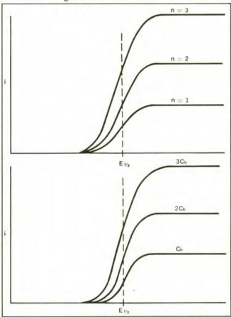
Figure 12. Effect of (a) n and (b) C<sub>b</sub> on the Limiting Current (other factors being constant).
