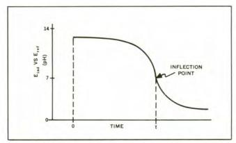
Figure 35. Coulometric Acid-Base Titration with Potentiometric Indication.
