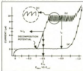
Figure 17. Polarogram of Cd++ in 1F HCl.
