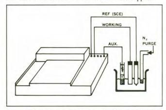
Figure 23. Instrumental Configuration for Chronoamperometry.
