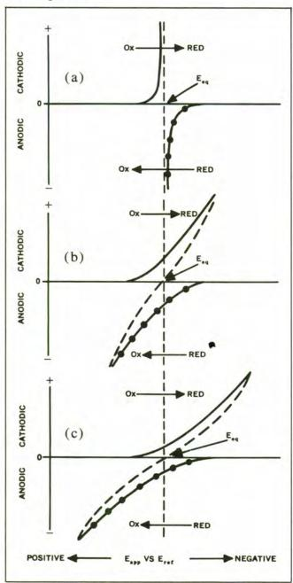
Figure 8. Idealized i-E Curve where (a) k, is Large, (b) k, is Small, and (c) k, is Very Small.
