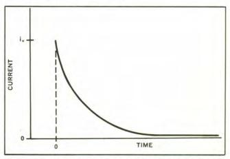
Figure 30. Typical i-t Curve for Controlled Potential Coulometry.
