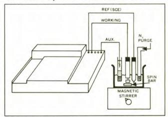
Figure 36. Instrumental Configuration for Electrodeposition and Separation.
