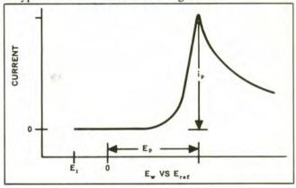
Figure 26. Typical i-E Curve.
