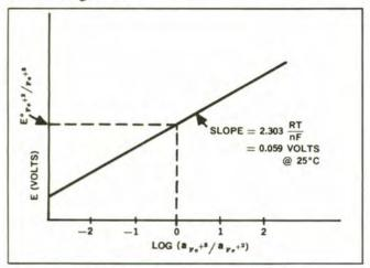
Figure 6. Plot of Potential Versus Log a<sub>Fe</sub>+3/a<sub>Fe</sub>+2.
