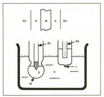
Figure 7. Schematic (a) and Physical Configuration (b) of pH Measuring System.  $R1 = Reference\ Electrode\ No.\ 1;\ R2 = Reference\ Electrode\ No.\ 2;\ S = Constant\ pH\ Solution;\ X = Unknown\ pH\ Solution;\ M = Glass\ Membrane;\ J = Liquid\ Junction.$
