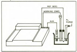
Figure 16. Instrumental Configuration for Polarography.
