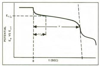
Figure 32. Typical Chronopotentiogram of the Reduction of Fe+3.
